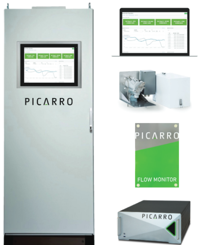
Figure 3. The Picarro EtO CEMS. State-of-the-art Picarro CRDS technology sits within a NEMA-12 (or better) industrial enclosure, with an umbilical connecting the system to the stack, where industry-leading flow monitoring and sample probes feed back essential parameters, and sample and calibration gases to enable real-time monitoring of both concentrations and mass emissions.
